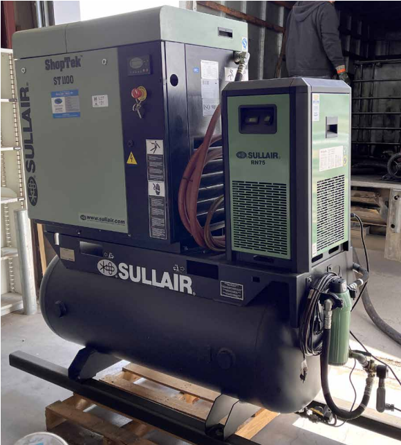
Sullair ST1109 Rotary Screw Compressor, Capture Tank, Dryer
