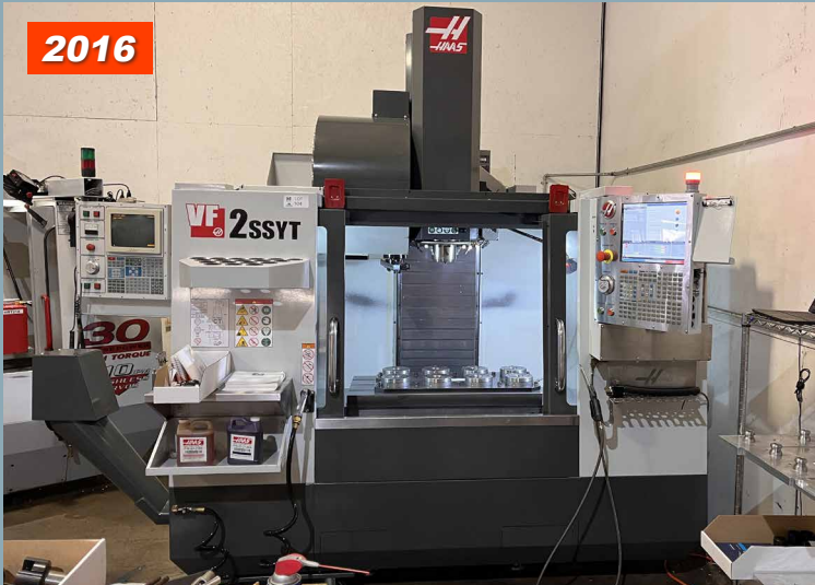
2016 Haas VF-2SSYT CNC Vertical Machining Center, New 2016, Through Spindle Coolant, 12,000 RPM, 24 ATC, Chip Auger, Tool Probe, Tool Setter, Manuals
