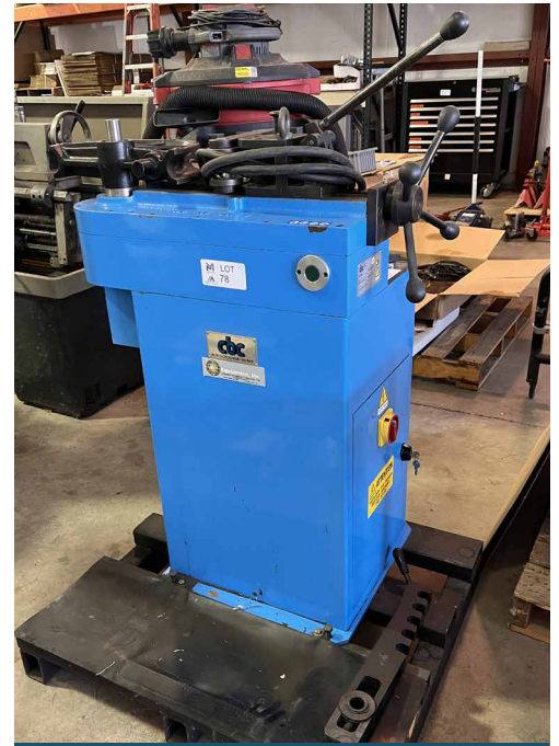
CBC UNI 70C Digital Pipe & Tube Bender, Misc. Dies
