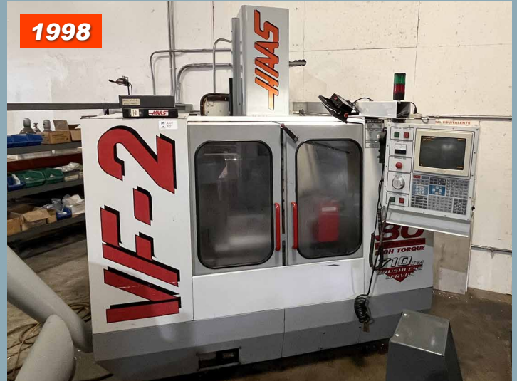
1998 Haas VF-2 CNC Vertical Machining Center, New 1998, 10,000 RPM, 20 ATC, P-Cool, Rigid Tapping, 4th Axis Ready, Chip Auger
