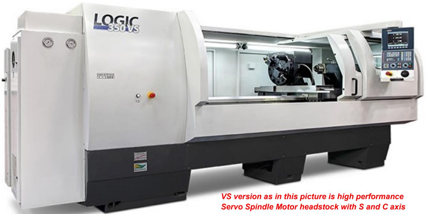
*VS version as in this picture is high performance Servo Spindle Motor headstock with S and C axis with live and dead tool turret for turning and milling*
