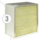
**3rd-Stage Fiber Filter:** 3rd stage Fiber Bed mist filter is depth loading that captures small mist particles. MERV 15\* filter rating.
