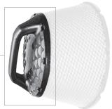
**1st-Stage Separation:** The coolant mist airstream initially collides with the fish scale profile coalescing the mist into larger droplets. Then, through a wind shear effect with the 70-degree, self-draining mesh filter, additional smoke and particles greater than 2 microns  $(2\mu m)$  are captured.
