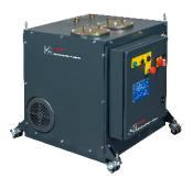
Chipblaster B-30/70 is a single M code controlled, fixed rate high pressure coolant system. The unit has 2 pleated, 10-micron filters that can be manually switched as needed, automatic overload system, and dirty filter alarm circuit. These features provide a safe machining process that helps prevent damage to the machine-tool, workpiece and tooling. Ideal for machine-tools up to 15 kW (20 hp) and 40 taper mills. The built-in casters make it easy to move for maintenance.
