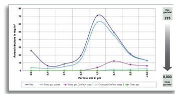
Example: Fraction separation degree of the Handte Oil Expert
