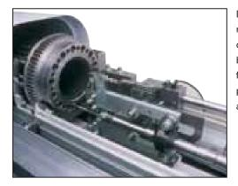
Double check remnant detection device speeds up bar end retraction for continuous production on all bar sizes.
