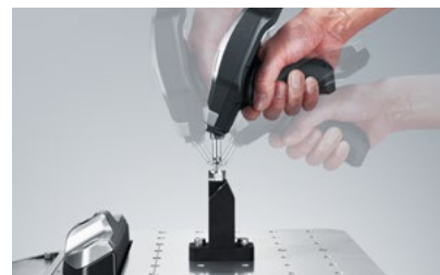
Easy calibration using the dedicated calibration jig
