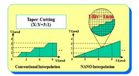
The Series 0i-MODEL TD achieves the highest precision possible with nanometer resolution standard throughout the CNC system - from internal calculations and stored values, through to the interpolator, on to the drive system, and the position feedback devices.
