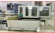
FOCUS PF-80H CNC AUTOMATIC CIRCULAR COLD SAW
