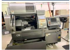
2005 CITIZEN C16 TYPE IX, S/N X13045, MITSUBISHI CINCOM CONTROL, 5/8" CAPACITY, 8 AXIS (INC. C1), 4 CROSS DRIVEN TOOLS, 6 OD, 6ID, 6 BW. **EQUIPPED WITH LNS THB 16-4.8 SINGLE TUBE BAR** FEED. THIS MACHINE IS NOT CURRENTLY RUNNING
