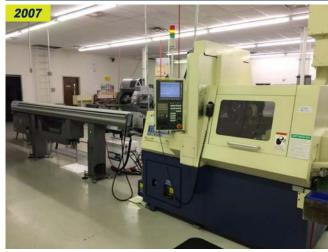
2007 TSUGAMI SS20 CNC SWISS LATHE, S/N 117. FANUC 31IT CONTROL, 3/4" CAPACITY, 7-AXIS (INC. C1), 24 TOOL POSITIONS, THREAD WHIRLER. EQUIPPED WITH TRACER MAGAZINE BF (SN 15070048), PARTS CATCHER, PART CONVEYOR, SIGNAL LIGHT, MP SYSTEMS 4-LINE HIGH PRESSURE COOLANT, TRIMIST MIST COLLECTOR
