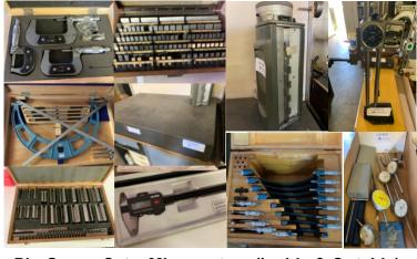
Pin Guage Sets, Micrometers (Inside & Outside), Calipers, Height Gages, Granite Surface Plates, Scales, Drafting Supplies, Broaching Sets, Dials, Parallels, Gage Blocks, Cylinder Gauges
