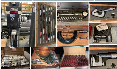
Pin Guage Sets, Micrometers (Inside & Outside), Calipers, Height Gages, Granite Surface Plates, Broaches, Dials, Parallels, Gage Blocks, Angle Blocks, Plug Gages, Bore Gages
