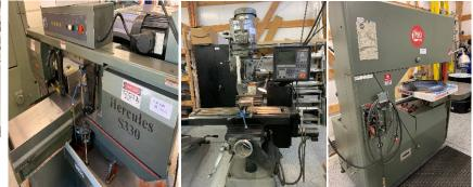
**Grob 4V-36 Vertical Band Saw:** 36", 5K FPM, 12" Work Height **Bridgeport Vertical Knee Mill:** 31"X, 12"Y, 16"Z, 4,200 RPM **Hercules S330 Horizontal Mitering Saw:** Capacity: 12" x 18", Blade Size: 13'6" W x .035" T
