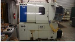
**Hurco TM6 CNC Lathe** Max Controls, 1.7" Bar Cap. 12-POS. Turret, 6K RPM Tail Stock. Parts Catcher. S/N 01003017AAA
